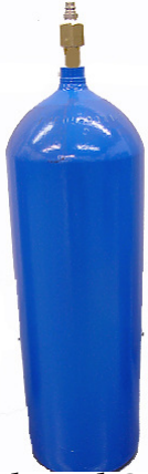
Calibrated Cylinder: Used to verify system accuracy on a daily basis
