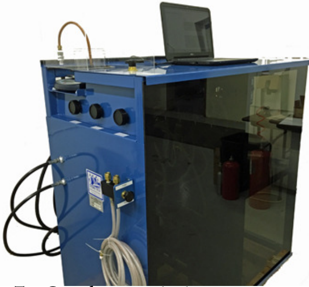
Test Console: Houses the electronics, pump, expansion device, valves, hoses, etc...
