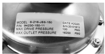
Typical label: "JBS" series rated to 16,000 psi
