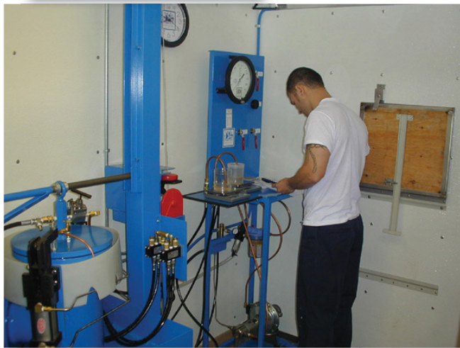
Model 500-2010 Small footprint test console with 10" dia. water jacket
