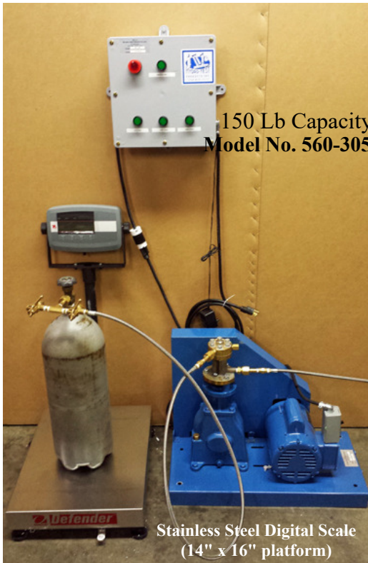
Model 560-305 Automatic Filling of 5-10-20 Lb. Cylinders
