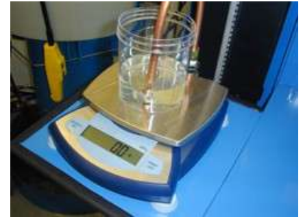
Expansion Device: A digital scale that is used to measure the expansion values of a cylinder under test pressure.
