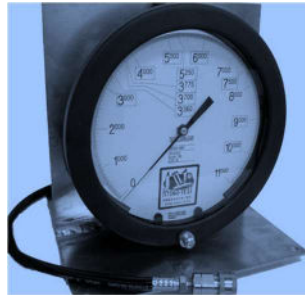
Dial Gauge: Used when operating the system in manual mode and to periodically calibrate the electronic pressure transducer
